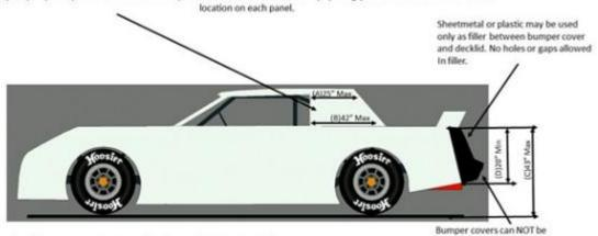
C-post (sail panels) Must be of the same shape and size on each side of car. Any openings/holes must be the same size and
